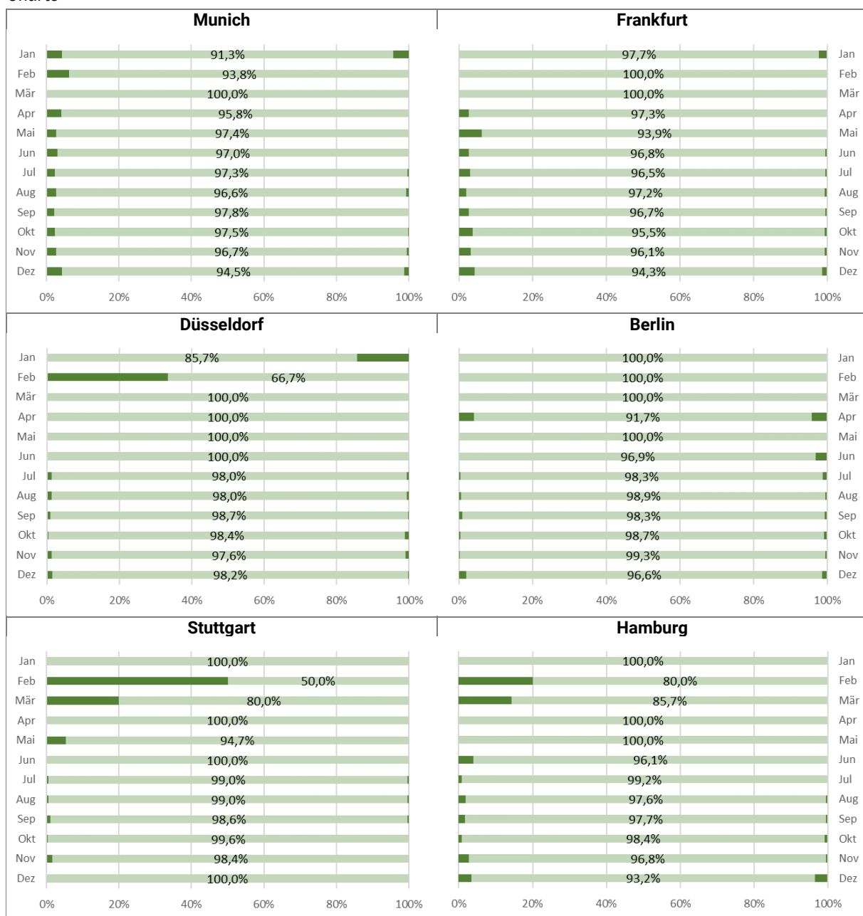
Fig. 9: Share of flights with ATOT before (dark green left), within (light green) and after (dark green right) STW
