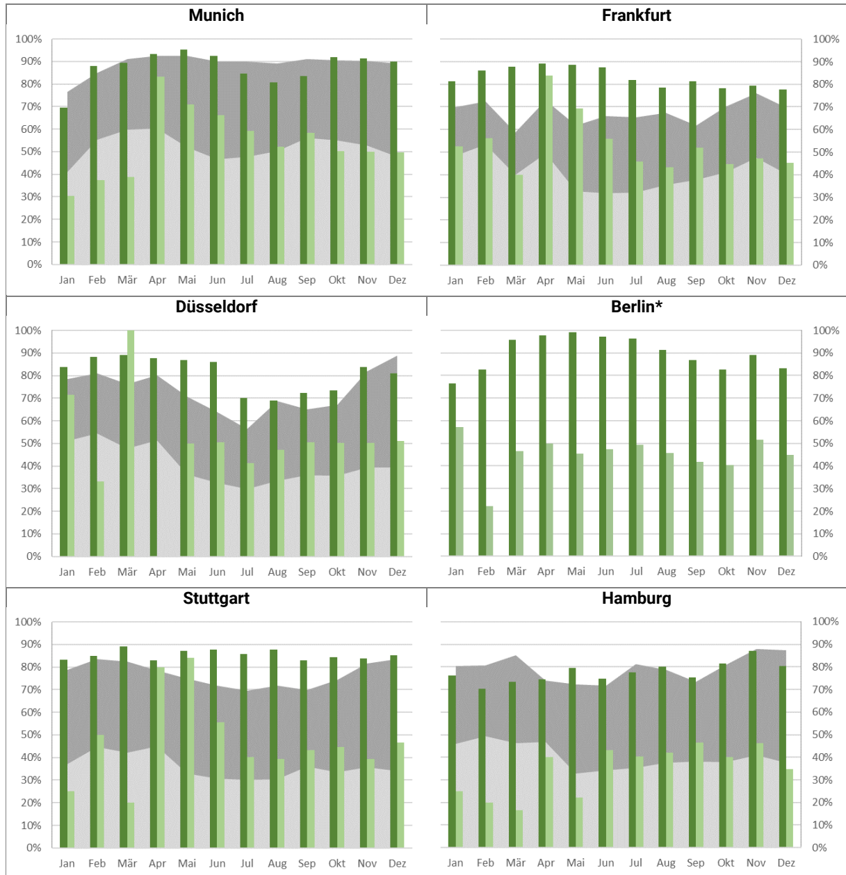
Fig. 3: Share of regulated and unregulated IFR departures 2020 (green) and 2019 (grey) where last TSAT = TOBT. Non-regulated flights in darker shade, regulated lighter.
